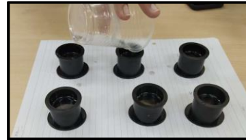
Figure 2: The Mixture Is Pour into Mould
