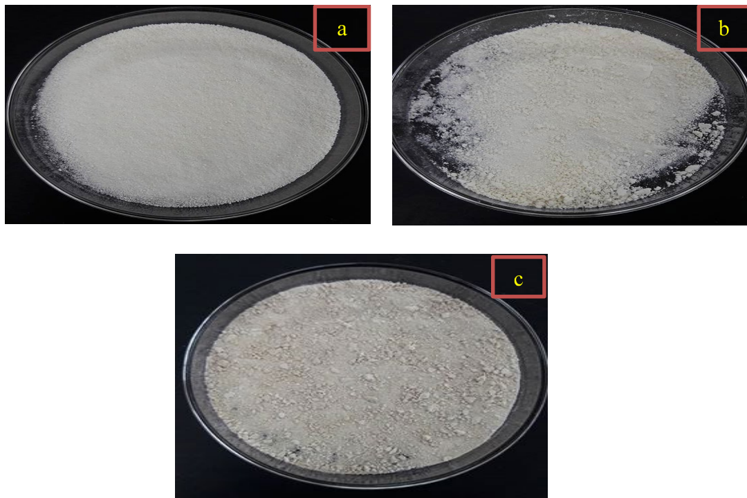
Figure 5: The colour appearance of (a) the Microcrystalline cellulose, (b) poly (AN-g-MCC) and (c) AO modified poly (AN-g-MCC).
