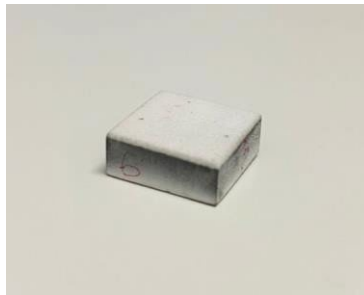
Figure 2: Specimen size: 15mm x 15mm x 6mm.
